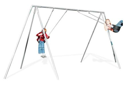
This is our shortest primary swing offered with the tripod support. This equipment is great for a smaller, controlled playground environment. Our 8 foot Primary Tripod Swings come with black cut-proof belt seats, 4/0 galvanized welded steel chain, and self-lubricating swing hangers. There are 2 seats per 10 foot section. The dimensions are as follows: 2-3/8" O.D. galvanized top rail, 1-7/8" O.D. galvanized legs, 8' installed height.
